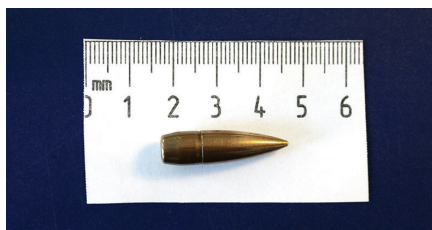
PHOTO 9.1 | The photo shows an unfired standard NATO bullet of the 7.62 x 51 mm full-jacketed type. Photo: P.Thiis Knudsen, Surg. Cdr RDNR.
