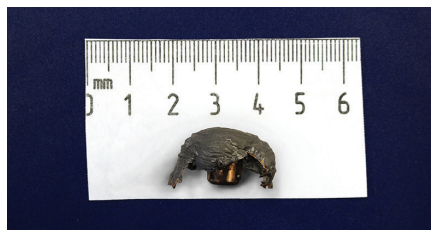
PHOTO 9.4 | The photo shows a fired expanding bullet of the 7.62 mm soft point type, that is the jacket does not cover the core and the lead, therefore, is visible at the tip. The bullet has been recovered from gelatine blocks. Photo: P.Thiis Knudsen, Surg. Cdr RDNR.
