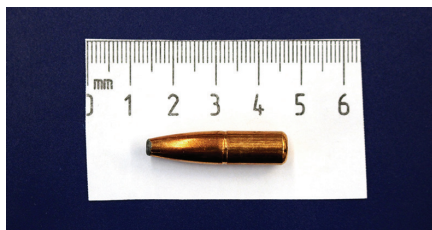
PHOTO 9.3 | The photo shows an unfired expanding bullet of the 7.62 mm soft point type, that is, the jacket does not cover the lead core, and the lead, therefore, is visible at the tip. Photo: P.Thiis Knudsen, Surg. Cdr RDNR.
