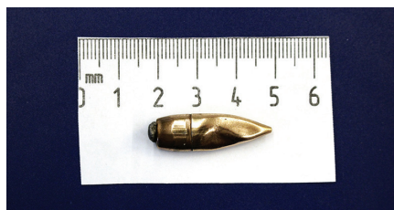
PHOTO 9.2 | The photo shows a fired NATO bullet of the 7.62 x 51 mm full-jacketed type. The bullet has been recovered from gelatine blocks. Photo: P.Thiis Knudsen, Surg. Cdr RDNR.
